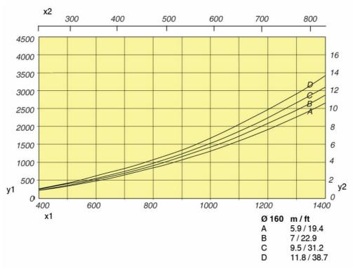
y1: Pressure drop (Pa), x1: Airflow (m3/h) x2: Airflow (cfm) y2: Airflow (in w.c)
